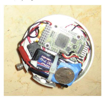
All connections to actuators and sensors are over an industrial serial bus, minimizing the weight and cost of the wiring. In addition with modern Lithium polymer batteries putting the battery at the point of load weighs less than the cabling that would be necessary to carry the power to an actuator.. Both of Unreasonable Rockets's flying vehicles from the LLC used this architecture.
