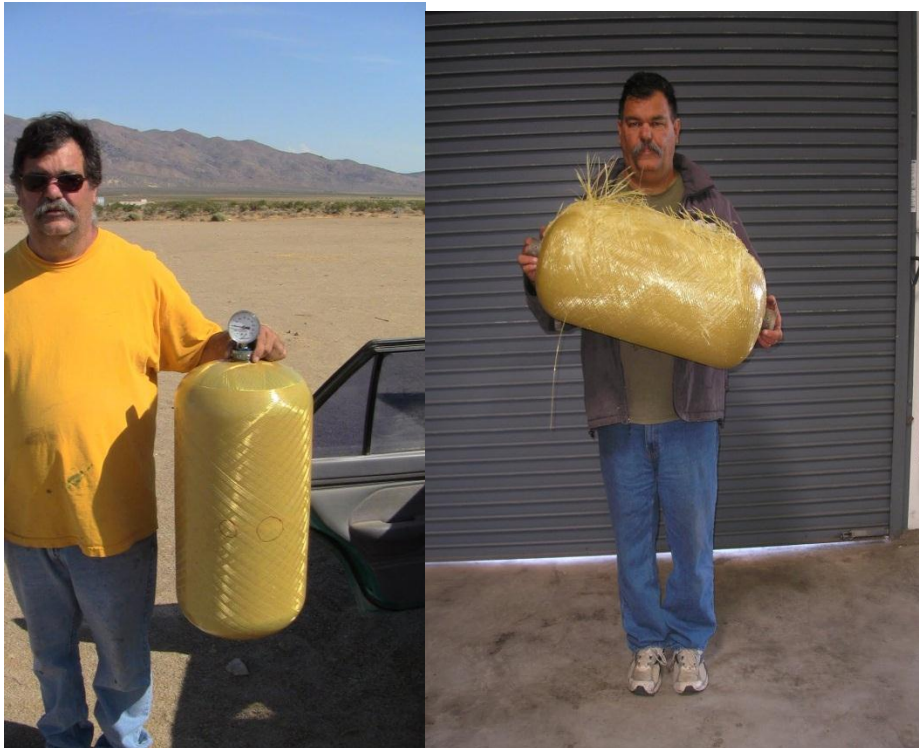
We have tested these tanks to failure and this failure matched our calculations.
